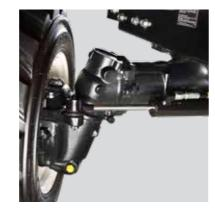
Hydraulic power steering Light steering makes the SA tractors easy to operate in confined spaces and helps minimise operator fatigue.
