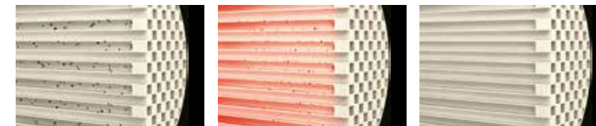
1. Particulate matter trapped 2. Regeneration starts 3. Regeneration completes*
